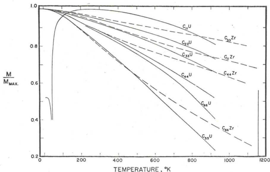
Fig. 5. Comparison of the temperature dependence of the principal stiffness moduli for alpha uranium and alpha zirconium<sup>10</sup>. Ordinate is the ratio of the modulus at temperature with respect to the maximum value of the modulus.
